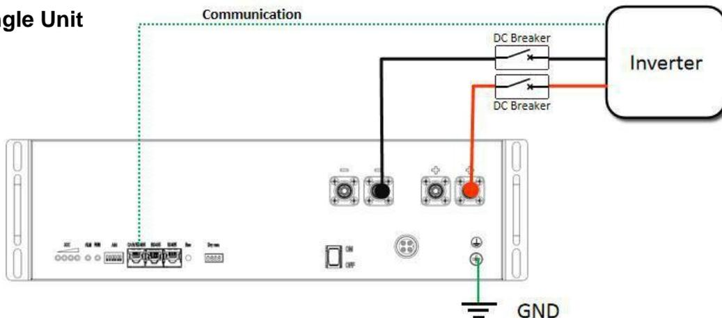
Figure 5 - Single Unit Connection
